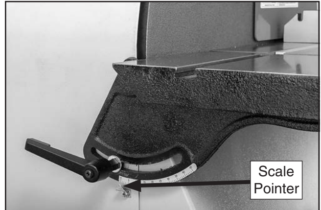
Figure 27. Scale pointer screw location.
